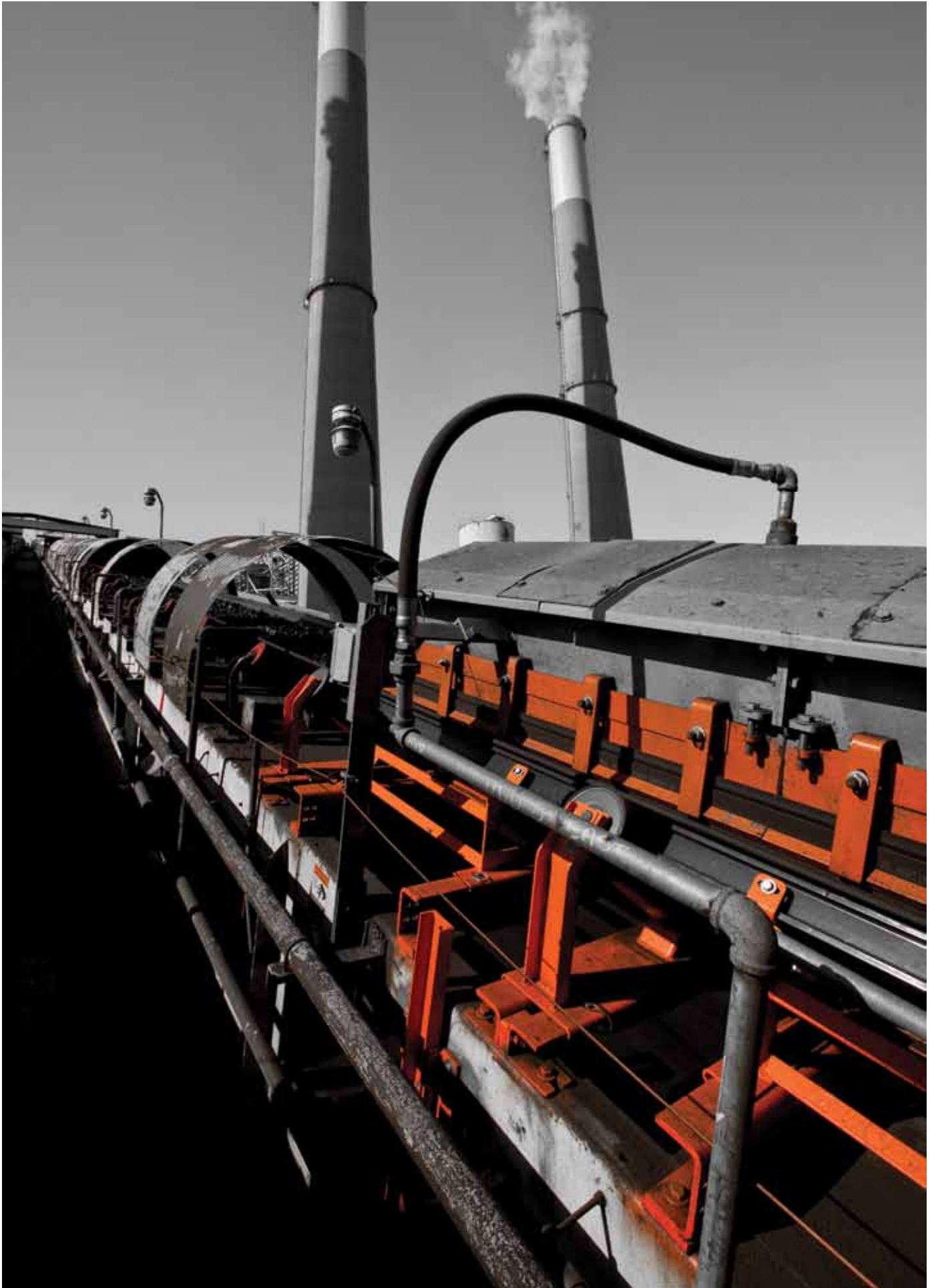
▲ Martin® Transfer Point Products stabilize the belt line and prevent spillage, while keeping the conveyor belt aligned.
